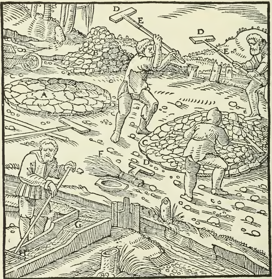
A—AREA PAVED WITH STONES. B—BROKEN ORE. C—AREA COVERED WITH BROKEN ORE. D—IRON TOOL. E—ITS HANDLE F—BROOM. G—SHORT STRAKE. H—WOODEN HOE.
